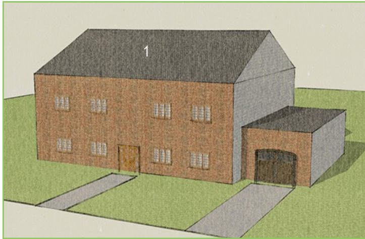
Figure 4.2.9.1 - Not Suitable - Only one (1) roof plane is visible from the public right-of-way.
